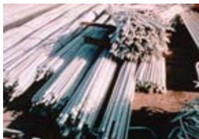
Standard-size reinforcing steel, both straight and fabricated, can be galvanized in advance and easily stored until needed.
